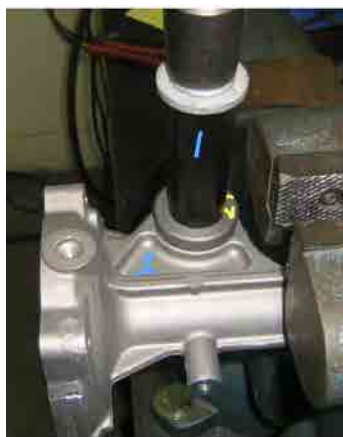
Figure 5 Outboard Housing Torque to failure set-up
