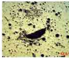
Fig.1.1: Shrinkage cavity, size 2.8 mm
