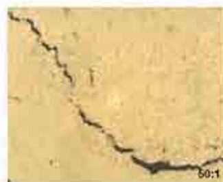
Fig. 1.1: Solidification crack , length 3,8 mm
