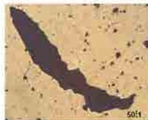
Fig.2.2: Shrinkage cavity, size 2.6 mm
