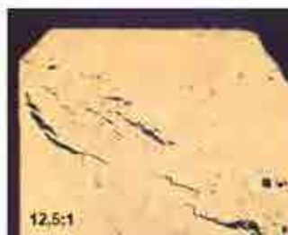
Fig.1.1: Continuous solidification cracks
